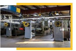
Multiple Spindle Screw Machines
